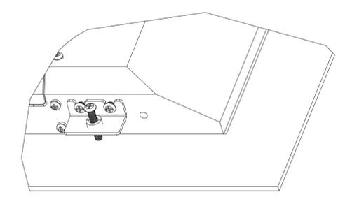
Step 4: Tighten the shorter M4x8mm screws to secure the bracket and tighten the longer M4x20mm screws to secure the monitor againstst the panel.
