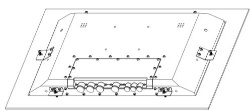
Step 3: Install the four remaining brackets. One on the left, One on the right, and two on top.
