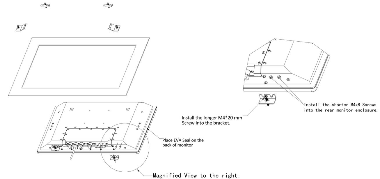
Step 1: Create panel cut out, place EVA seal, and install two bottom brackets.
